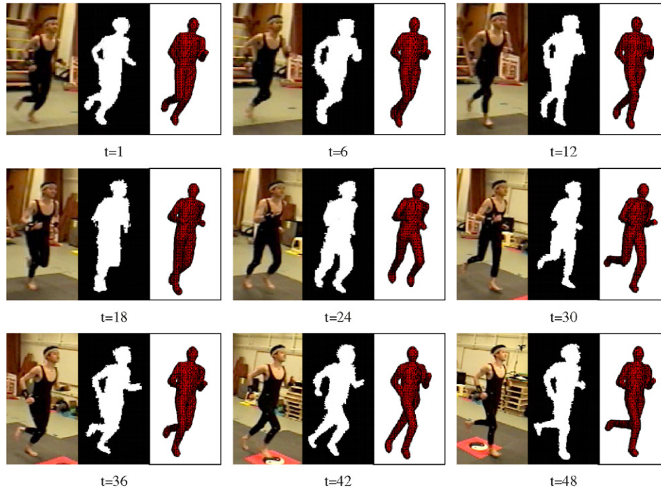
Fig. 14. Results of 3D human pose reconstruction from an image sequence in which a subject is performing a running motion. The images are extracted from the video taken from the web site http://mocap.cs.cmu.edu/ .
